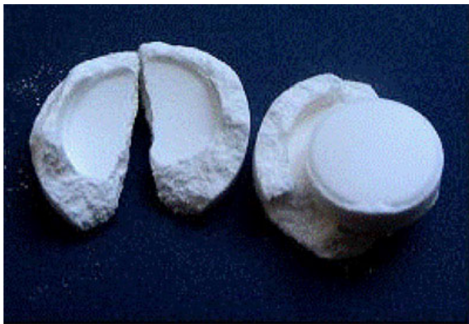
Figure 2. Equatorial fracture showing the surfaces of the compressed ethylcellulose core tablet system.
